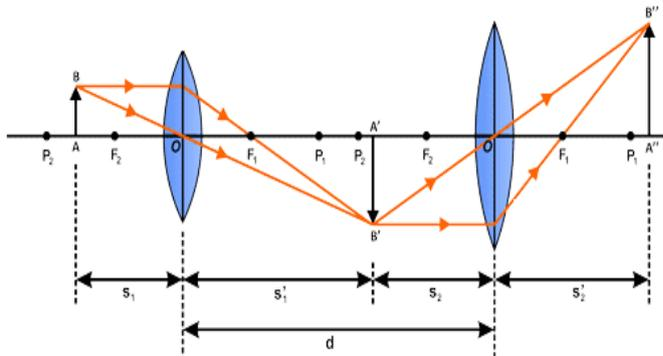
**Figure 3 : Microscope**
